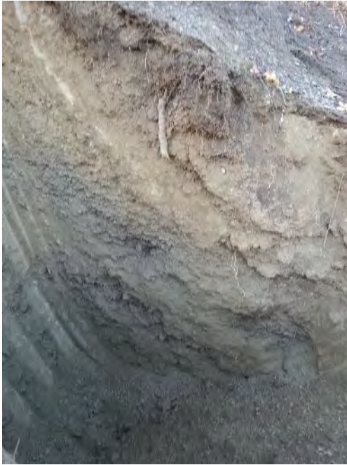
Photo 1: Test Pit 2 indicating surface topsoil and the gravelly SILT/SAND subsurface material.
