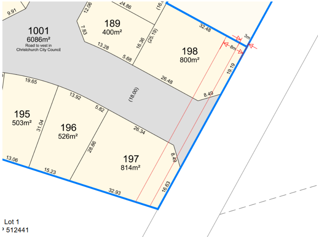
Figure 3 3m landscape strip and 8m building setback as shown on lots 197 and 198
