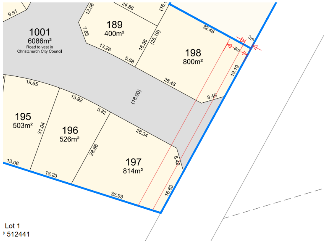
Figure 4 3m landscape strip and 8m building setback as shown on lots 197 and 198
