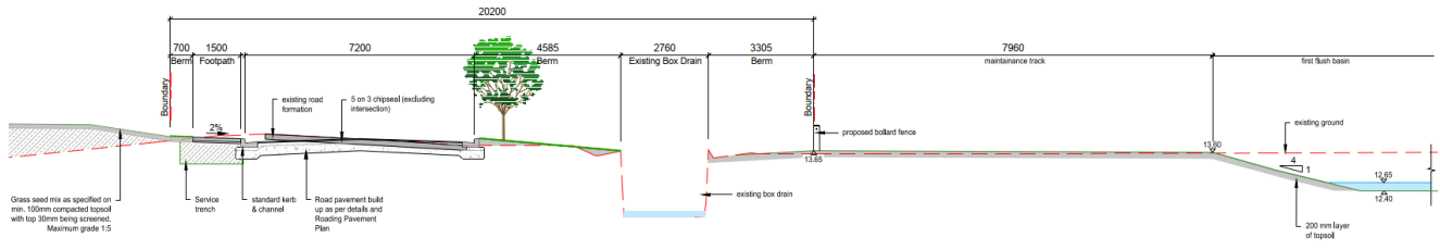
Typical Cross-Section - Hawkins Road '2-2' Scale 1 in 100
